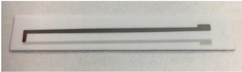
Figure 12 Stencil printed ITON/Pt thin film thermocouple on alumina substrate [65]
