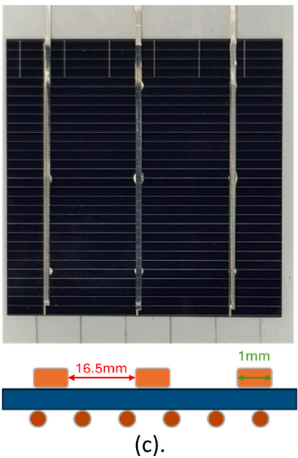
Fig. 3. Photos and schematic cross-section of the test devices, a) DWB solar module with a magnified view of a connection pad, b) Solar module with 6 tabbing wires on both sides, equivalent M2+ solar module with 18 tabbing wires and c) Solar module with 3 tabbing ribbons on the front side, equivalent M2+ solar module with 9 tabbing ribbons.
