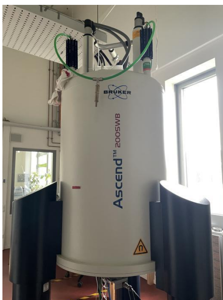
Figure 16. The NMR spectroscopy measurements in this study were performed on a Bruker Ascend 200SWB, operating at 600 MHz.
