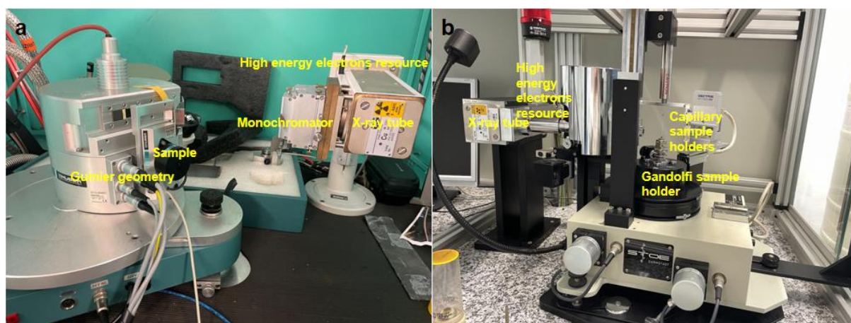
Figure 10. Construction and important components of the xHuber from JCNS-2 Lab (a) and STOE from the Inorganic Chemistry Lab, University of Cologne (b).
