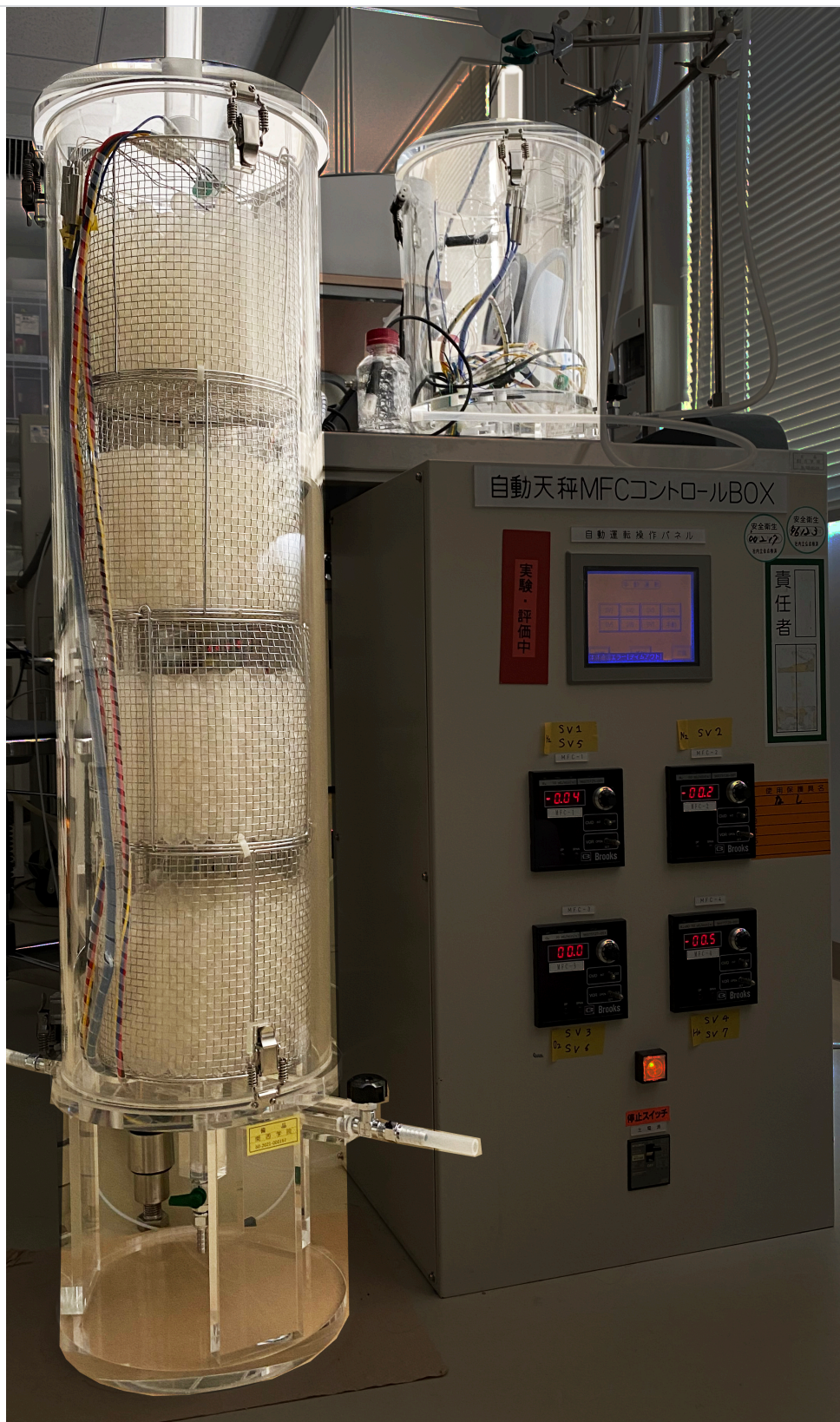
Figure 2. A prototype full-sized transparent storage canister "REKO-T" filled with simulated fuel debris
