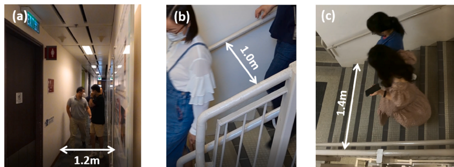
Fig. 8. Evacuation flows in corridors and staircases.
