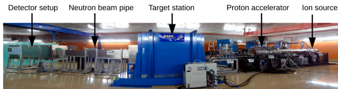
Fig. 7.1. RANS facility showing relevant components for a CANS: Accelerator, target station, instrumentation.
