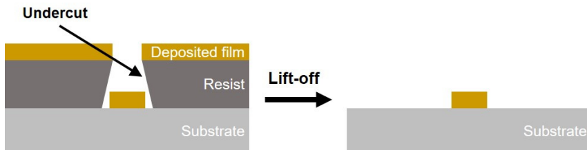
Figure 6.7: Schematic diagram of undercut resist profile for lift-off patterning.
