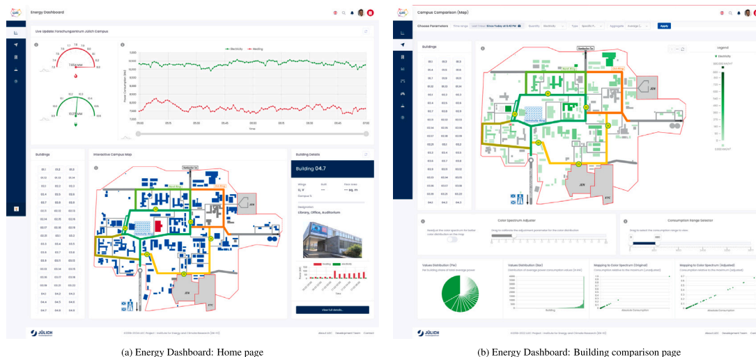
Fig. 4. Screenshots of the Energy Dashboard. (a) Exemplary building page showing live electricity and thermal demands. (b) Comparison of building thermal demands in a map-based view.
