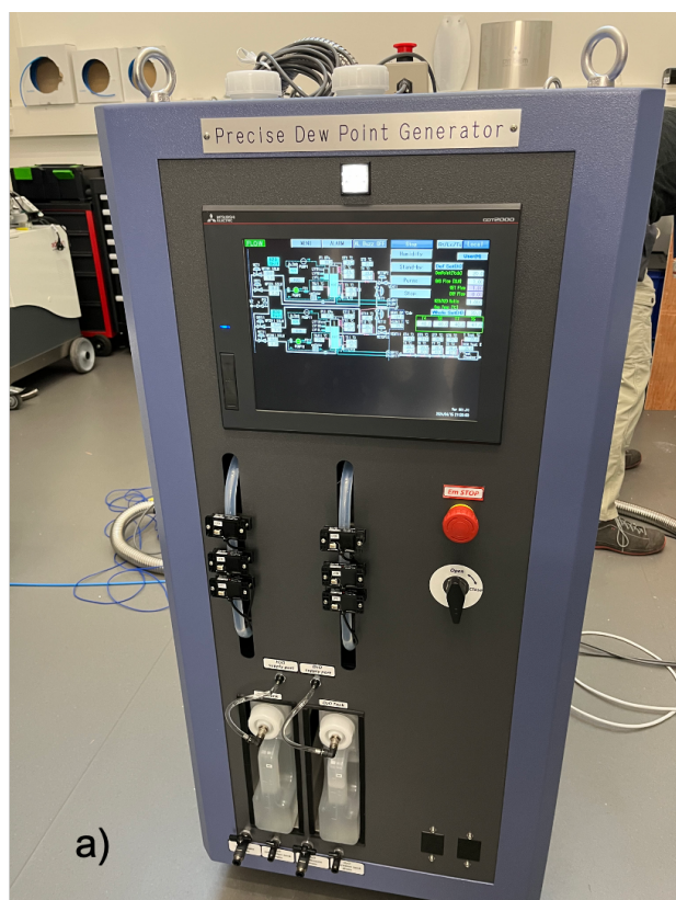
Figure S3 The precise dew point generator with two reservoirs for in-situ changing the contrast in the sample by providing vapor of either H 2 O, D 2 O or any H 2 O/D 2 O combination (left) and the multiposition sample chamber that works together with the generator. The dew point mirror sensor setup is visible in top of the chamber. Photos are taken during the calibration test carried out at JCNS.
