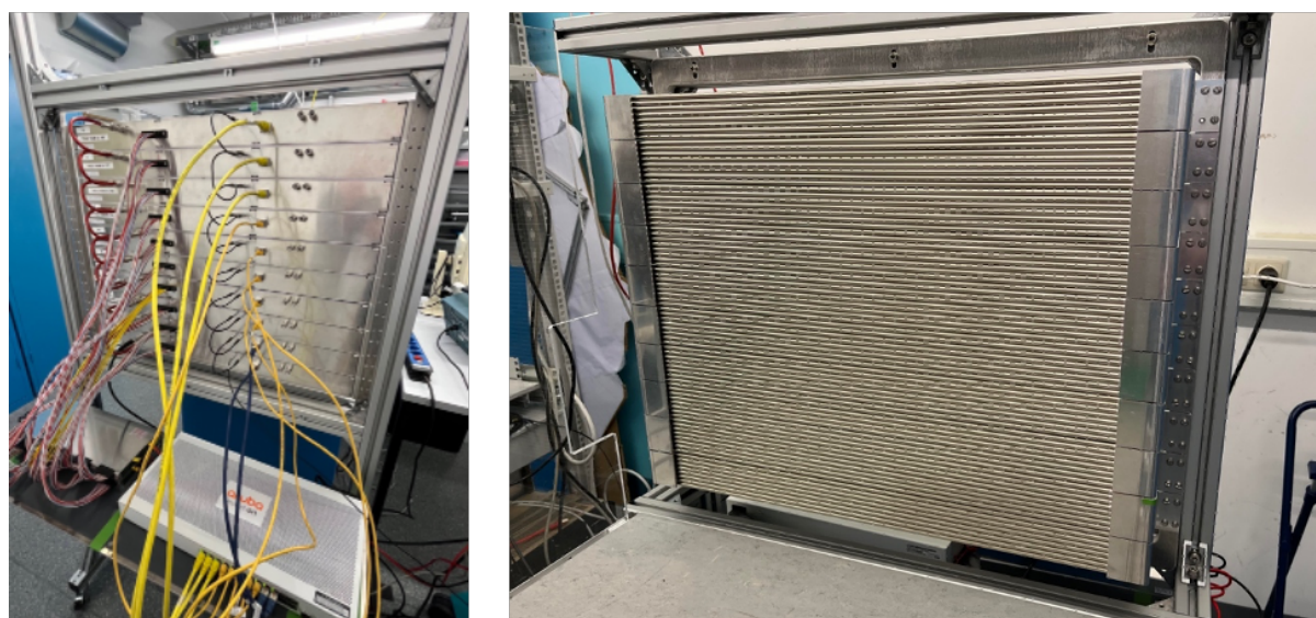
Figure S8 The ^3\text{He} detector tubes array during the test with the ^{252}\text{Cf} source at FRM II, MLZ Garching: the backside of the detector with the signal and power cables (left) and the front side (right).
