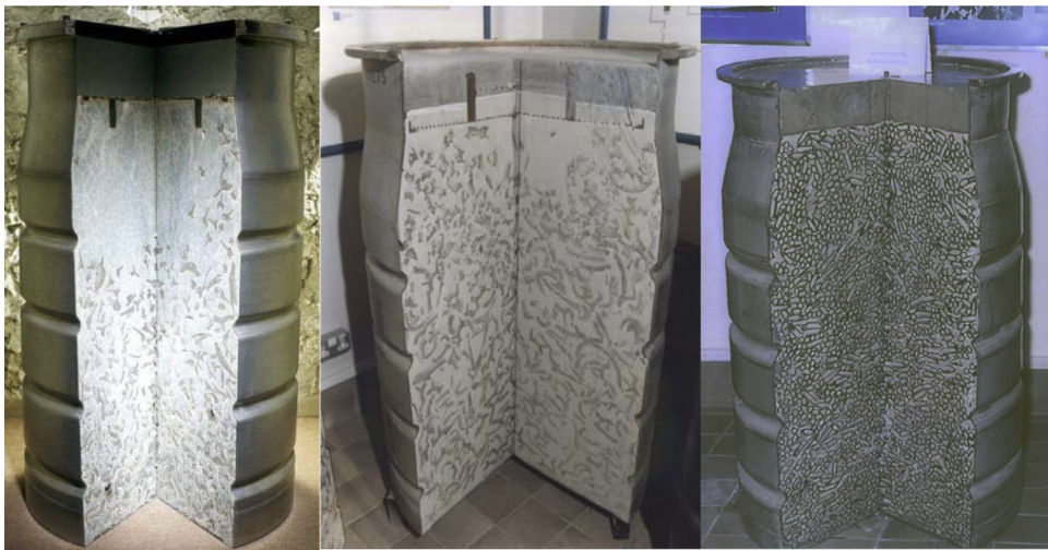
Figure 2.9: Drums containing solid, liquid and slurry intermediate-level waste immobilized with cement [Ojo05, p.226].
