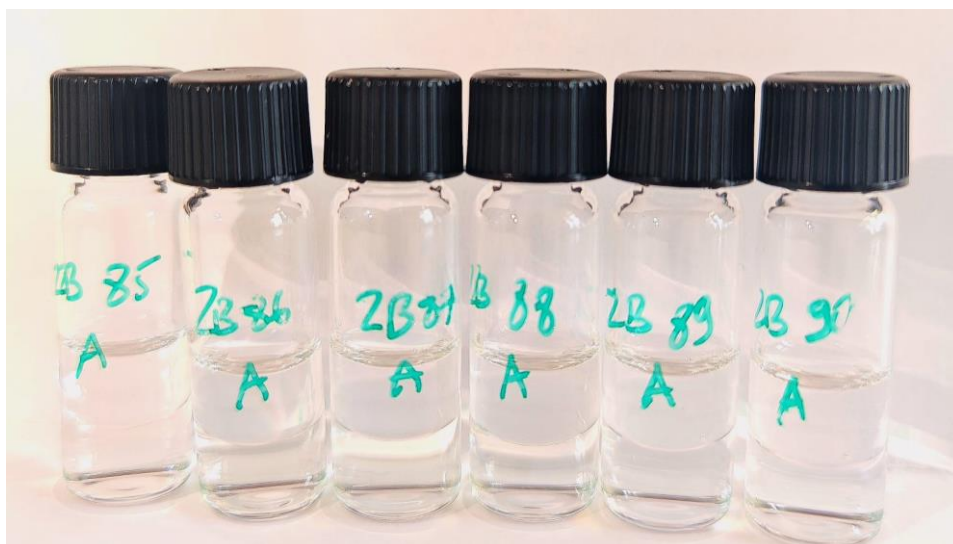
Figure 24: Samples after centrifugation, extraction series with 0.02 mol/L PTD in nitric acid. Organic phase: 0.2 mol/L Me-TDDGA in n -dodecane. Aqueous phase: 0.02 mol/L \text{SO}_3\text{-Ph-BTP} , 0.052 to 3.38 mol/L \text{HNO}_3 , 10^{-5} mol/L Ln(III) (without Pm and Y) and ^{41}\text{Am} , ^{244}\text{Cm} , ^{152}\text{Eu} , ^{239}\text{Pu} , ^{237}\text{Np} , U-nat, T = 22^\circ\text{C} \pm 1^\circ\text{C} , mixing time t=30 min.
