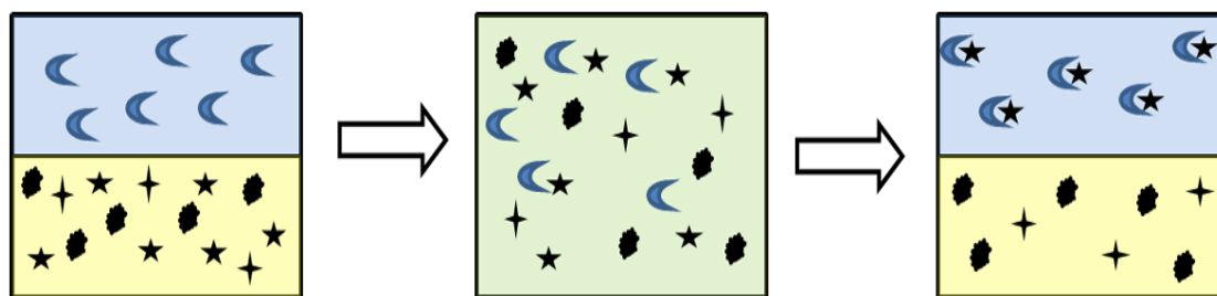
Figure 1: Solvent extraction process explained, an organic solvent (blue) with extractant molecules (blue symbols) is mixed with an aqueous phase (yellow) containing metal ions (black symbols) to maximize contact. After phase separation, the extracted ions transfer into the organic phase [6].
