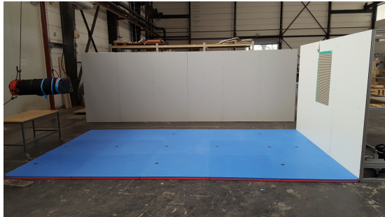
Figure 1: The Experimental area covered with mats has a size of 3\text{ m} \times 5\text{ m} . On the left side, a punching bag was suspended from the ceiling to push the participants forward. The right side of the area was limited by a solid wall.
