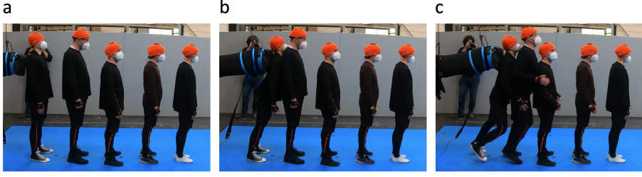
Figure 1: Snapshots of the experiments from the side-view camera. Five people lined up along the y-axis in front of a punching bag. (a) At the beginning of the trial, all participants stand at rest. (b) The last person in the row is pushed forward by the punching bag and touches the next person. (c) The impulse reaches the third person of the row.
