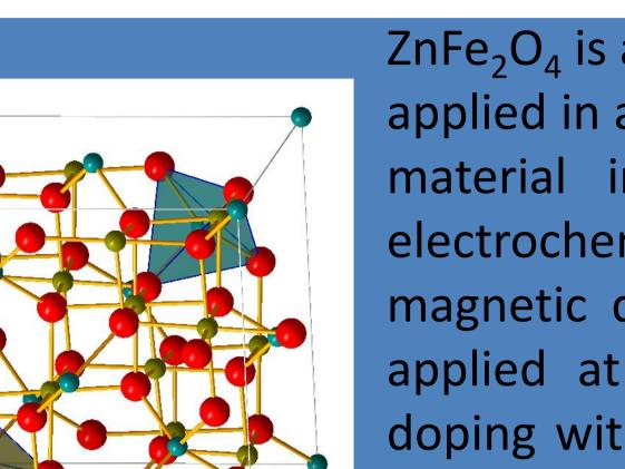
ZnFe<sub>2</sub>O<sub>4</sub> is a well-known spinel material which is applied in a variety of areas ranging from anode material in lithium-ion batteries to photoelectrochemical water splitting and high-density magnetic data storage [1], but it can also be applied at the cathode in zinc batteries. By doping with a non-redoxactive cation on the B position (Al<sup>3+</sup>), we tried to improve cycling stability and prevent Fe leaching in contact to aqueous electrolytes.
