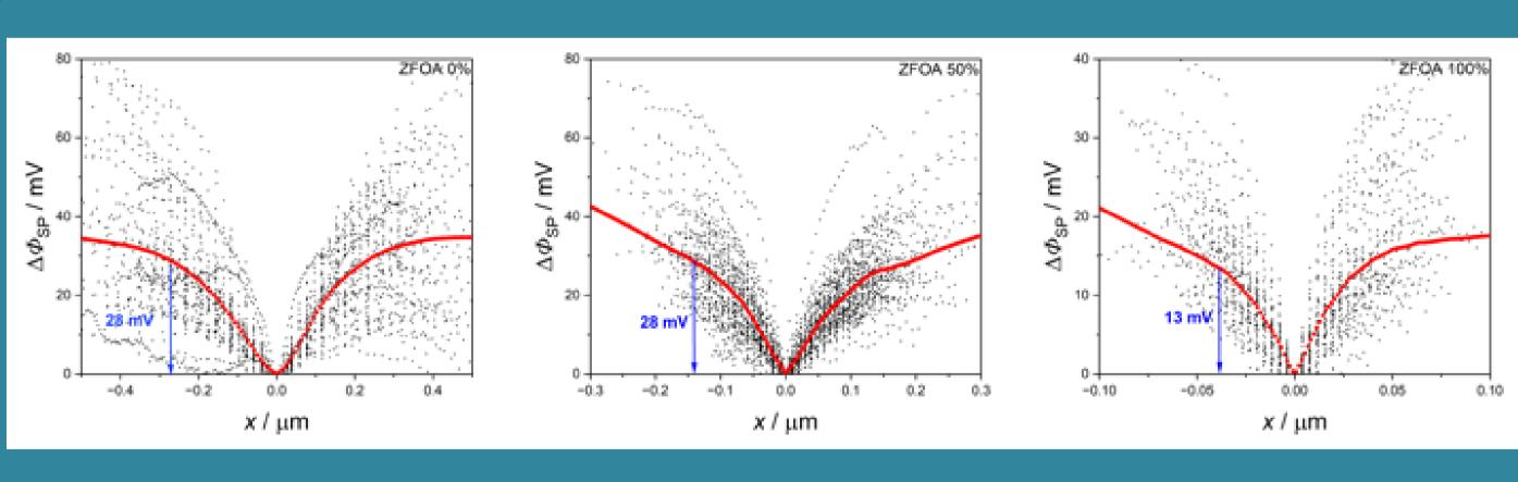
AFM measurements in accordance to impedance spectroscopy measurements show that Al concentration does not affect the potential barrier at the grain boundaries
