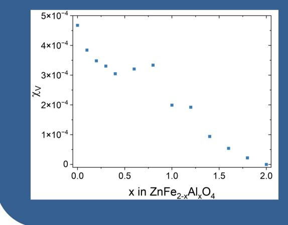
Magnetic properties change strongly: pure Gahnite is diamagnetic, pure Franklinite can be picked up with a magnet
