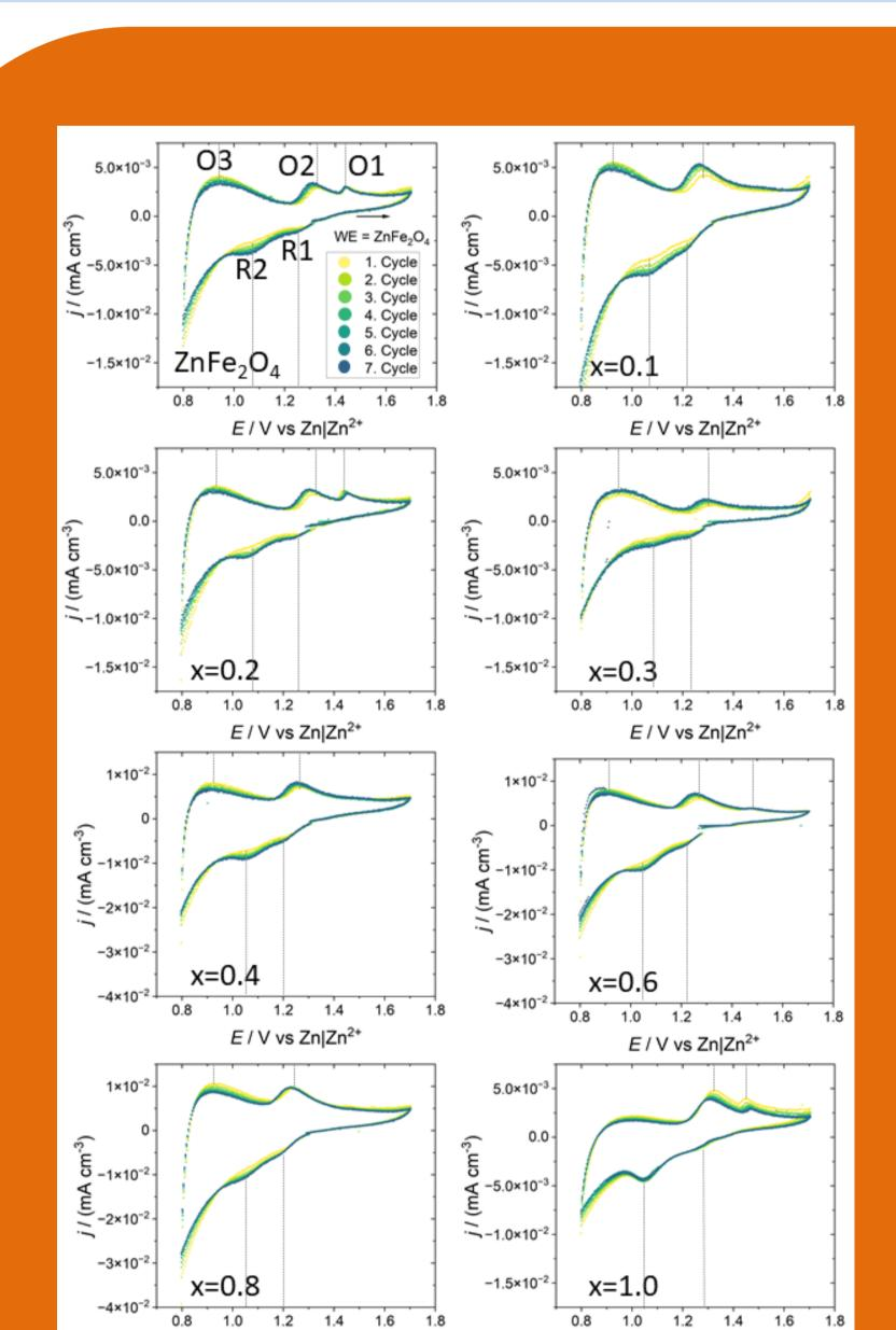
All materials up to x=1.0 show reversible Zn<sup>2+</sup> (de)insertion (O2/R2) and additionally more or less pronounced proton (de)insertion (O1/R1).
