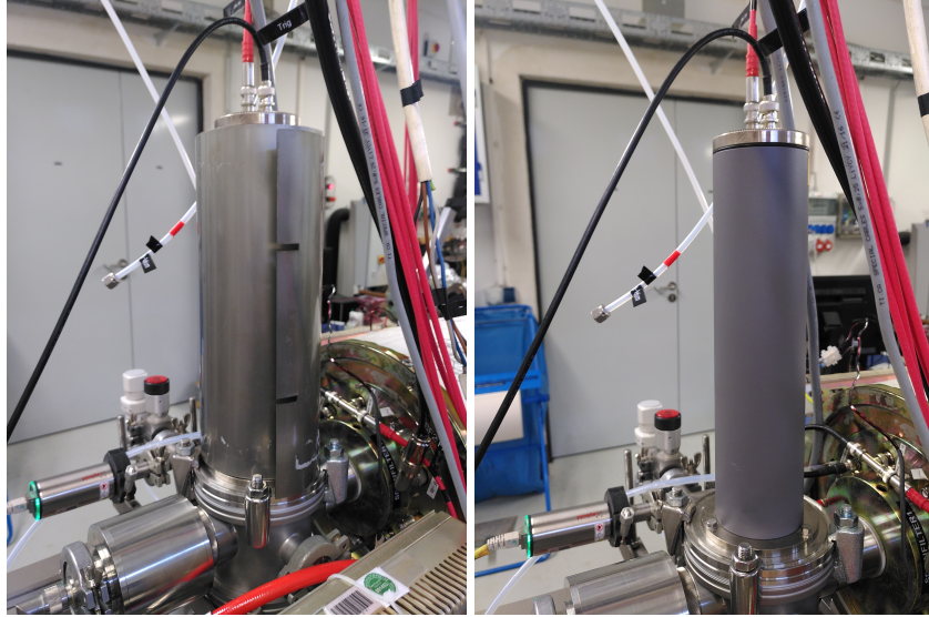
Figure 19: Photomultiplier (PMT) with (left) and without (right) magnetic shielding.
