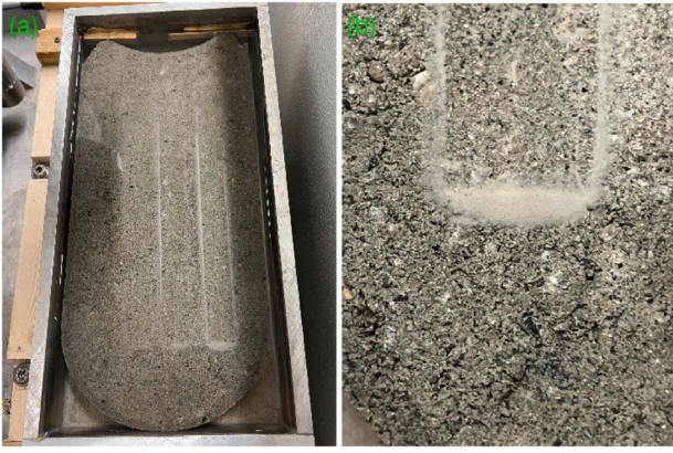
Fig. 6. (a) Wear tracks for the silica-filled SBR block sliding on a “smooth” concrete surface in water. The sliding motion consisted of 10 sliding cycles, each comprising a 20 cm forward and backward motion. (b) Magnified view of the wear particles accumulated at the edge of one sliding track.
