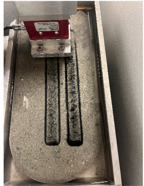
Fig. 5. Wear tracks for the carbon-filled SBR block sliding on a “smooth” concrete surface in water. The sliding motion consisted of 10 sliding cycles, each comprising a 20 cm forward and backward motion.
