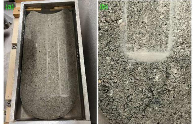
FIG. 6. (a) Wear tracks for the silica-filled SBR block sliding on a “smooth” concrete surface in water. The sliding motion consisted of 10 sliding cycles, each comprising a 20 cm forward and backward motion. (b) Magnified view of the wear particles accumulated at the edge of one sliding track.
