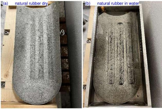
FIG. 11. Wear tracks for the carbon-filled NR block sliding on a concrete surface in water. The sliding motion consisted of 10 sliding cycles, each comprising a 20 cm forward and backward motion.
