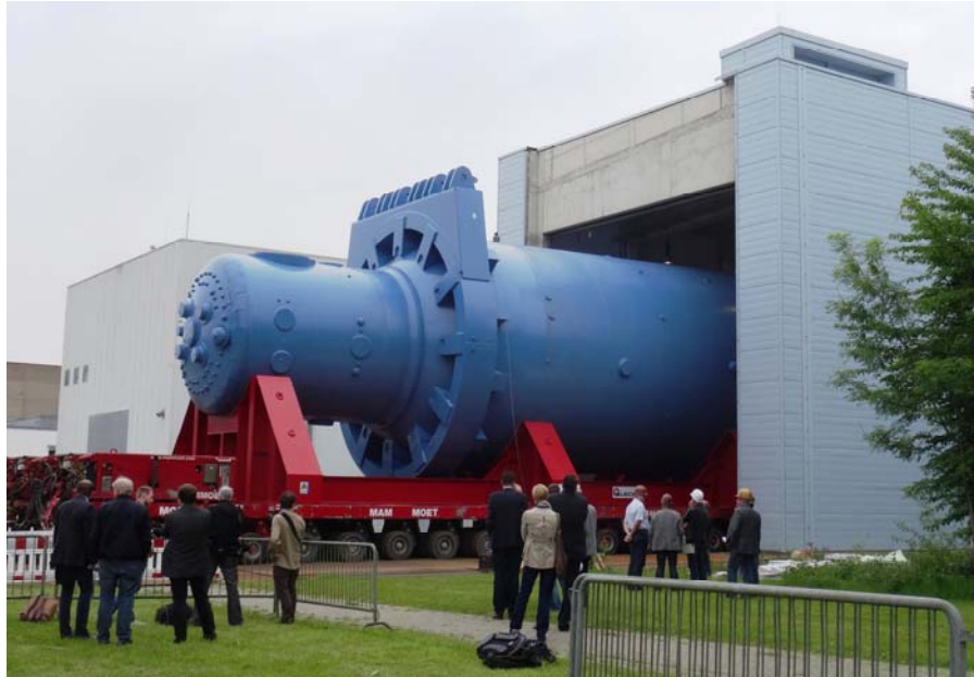
FIG. 3. Transport of AVR reactor vessel to interim store.
