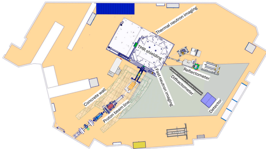
Fig. 1. The sketch of the JULIC neutron platform. The heavy concrete wall around the proton beam tube in a partially transparent green color.
