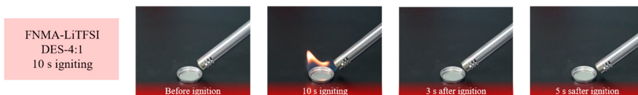
Figure 4. Photographs of flammability test of liquid DES-4:1, which was ignited under open flame for 10 s.
