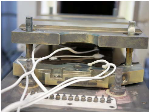
(a) Experimental arrangement for contact resistance tests
