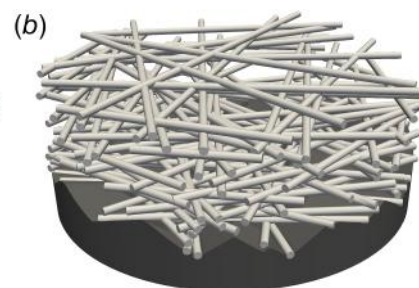
Fig. 1 (a) Sketch of the MPL creation. A pure MPL layer is present below the fiber substrate. In the intermediate layer, both fibers and MPL are present. The MPL intrudes into the pores of the fiber substrate. Areas above fibers are left empty. The slope of the MPL intrusion into the fiber substrate pores is given by the angle \alpha . (b) Simulation domain of fibers on the top and MPL on the bottom. The fibers are discretized in 1D along the fiber direction. The MPL is discretized into 3D polyhedral cells.
