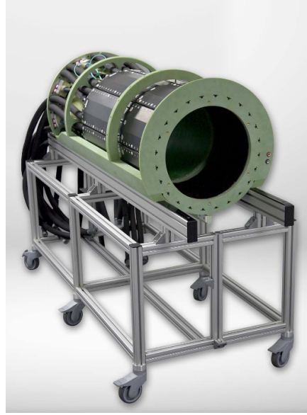
(a) BrainPET 7T insert without cover and RF coil array on installation cart.
