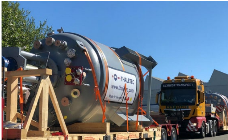
Image: THALETEC GmbH – BE-type enameled mixing tank with a volume of 16,000 l – www.thaletic.com
