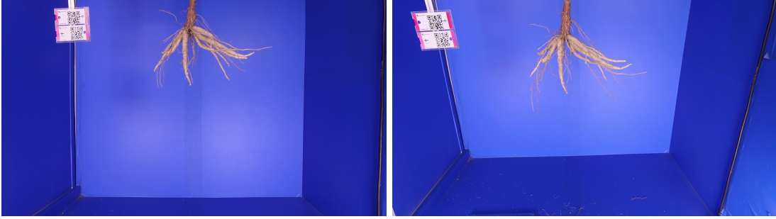
Figure 5: Sample stereo image pair from the 9-week cassava root example reconstruction (frame 0 from each camera). Left: lower camera view. Right: upper camera view. The two cameras are mounted with a 30 cm vertical baseline, capturing synchronized frames during 360° rotation.
