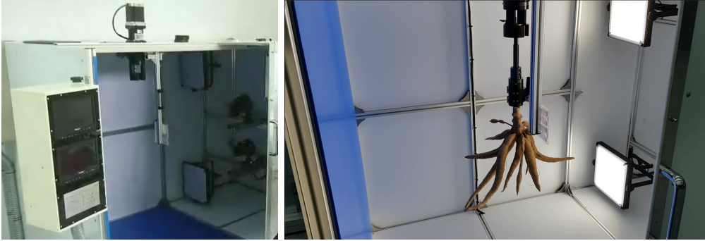
Figure 3: Setup features a closed environment with a vertically-aligned stereo imaging system, and a holder for the cassava plant, allowing it to rotate 360 degrees in 6 seconds.
