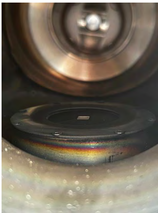
Figure A.15.: Position 0. No target positioned above the substrate/sample in the heater block.
