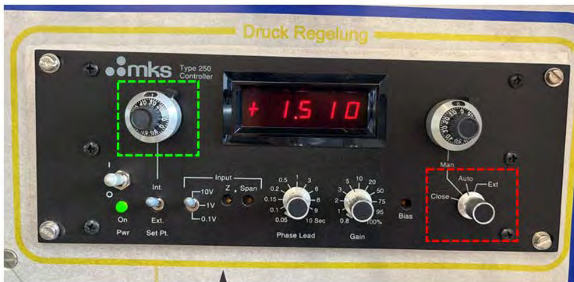
Figure A.20.: Vacuum measurement and MKS panel. Follow the instructions to insert oxygen into the chamber under a controlled value of pressure.
