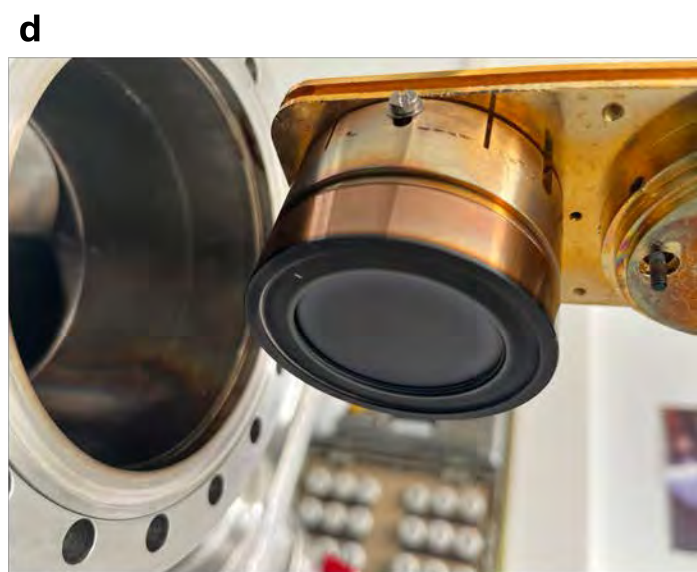
Figure A.33.: (a-c) Connect the structure to the target arm by tightening the screws. (d) If necessary, tighten up the bottom part of the external structure of the target to have it more adjusted.
