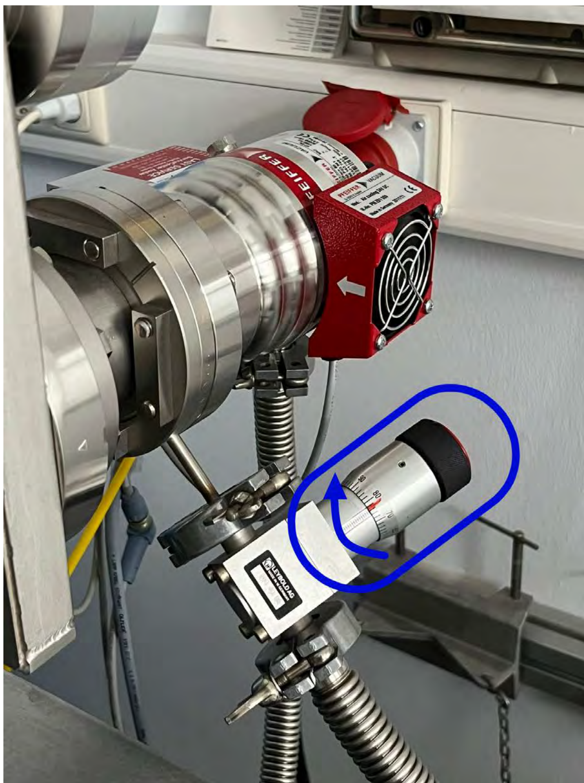
Figure A.21.: Remember to close the bypass valve for sputtering experiment with pressures bigger than 2.25 mbar.
