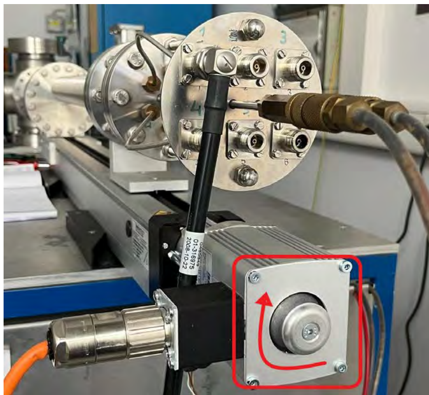
Figure A.16.: Rotate clockwise to move forward a desired target to the deposition position. Rotate counter-clockwise to return the target back.
