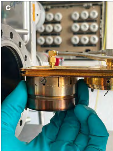
Figure A.33.: (a-c) Connect the structure to the target arm by tightening the screws. (d) If necessary, tighten up the bottom part of the external structure of the target to have it more adjusted.
