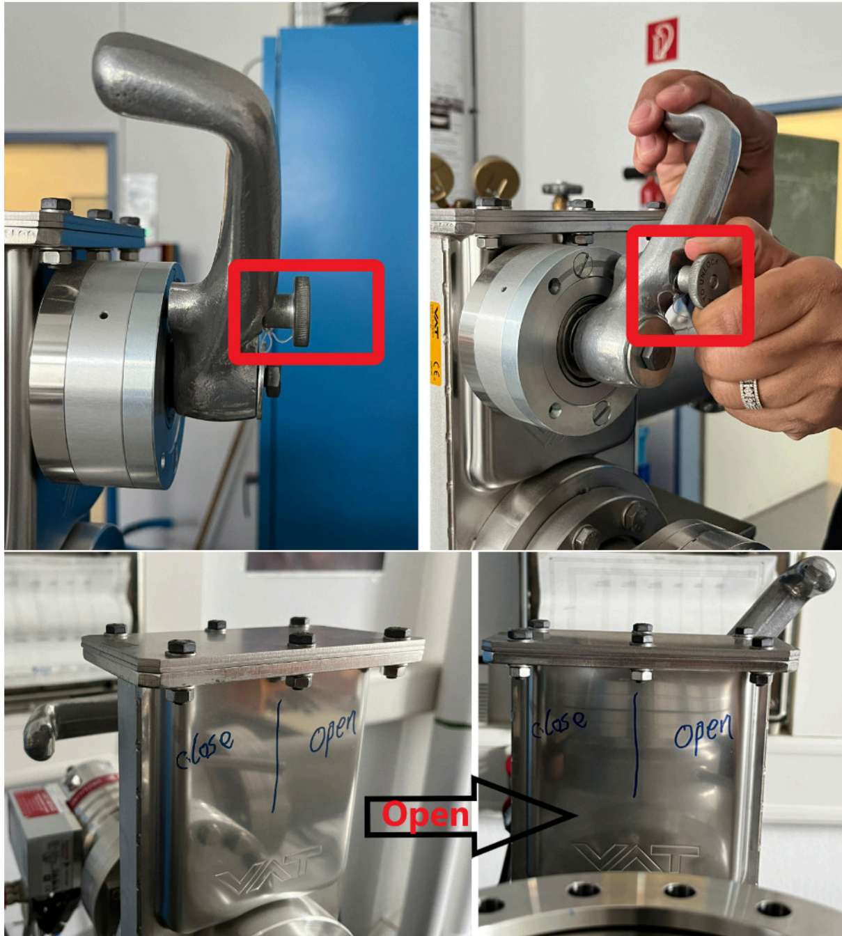
Figure A.11.: Opening the gate valve: pull the pin and turn the valve to the right. Lock it with the pin.
