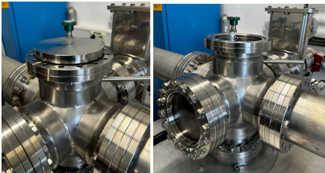
Figure A.8.: Chamber lid without the external ring and open.
