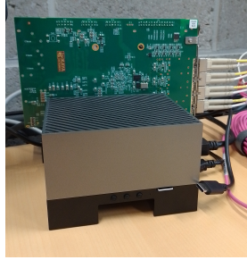
Fig. 1: The edge device, an Nvidia AGX Orin (front), with a frame grabber PCIe card (green) for interfacing with high-speed cameras over fiber.
