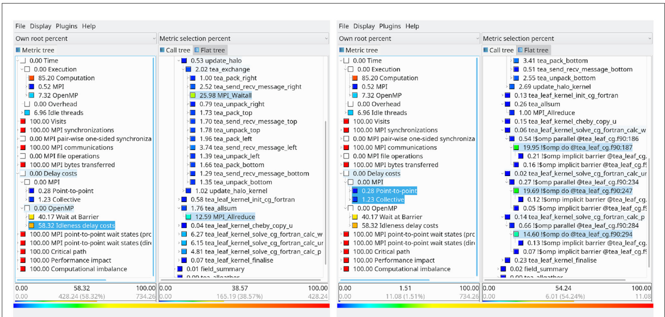
FIGURE 8 Screenshots of a Scalasca Trace Tools analysis result in the CubeGUI, showcasing the root cause analysis. (Left) MPI communication times and related wait states are negligible (0.52% of the overall run time; see MPI sub-metric in the Time metric tree at the top of the left pane). However, a significant proportion of the OpenMP thread idleness (selected node in the Delay costs metric tree in the left pane) is caused by data exchanges, that is, the MPI communication calls highlighted in the call tree (right pane). Thus, even minimal improvements can have a significant impact. (Right) The delay costs of MPI wait states (selected nodes in left pane) are caused by computation and load imbalance in the OpenMP-parallelized solver loops (highlighted call paths in the right pane), delaying subsequent communication operations. That is, inefficiencies in the solver loops cause cascading effects, amplifying their importance on overall performance.
