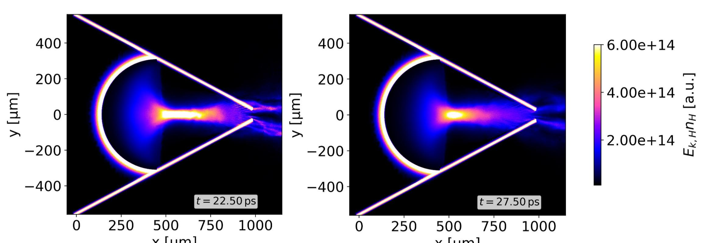
\*\* Simulations performed in pFI conditions:  $2 \times 10^{19} \text{ W} \cdot \text{cm}^{-2}$ , 1.8 ps,  $D_L = 640 \mu\text{m}$
