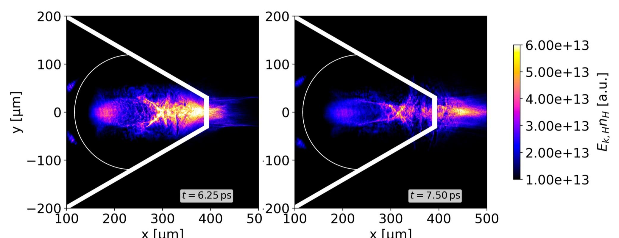
\* Simulations performed for OMEGA-EP parameters:  $7 \times 10^{19} \text{ W} \cdot \text{cm}^{-2}$ , 700 fs,  $D_L = 35 \mu\text{m}$
