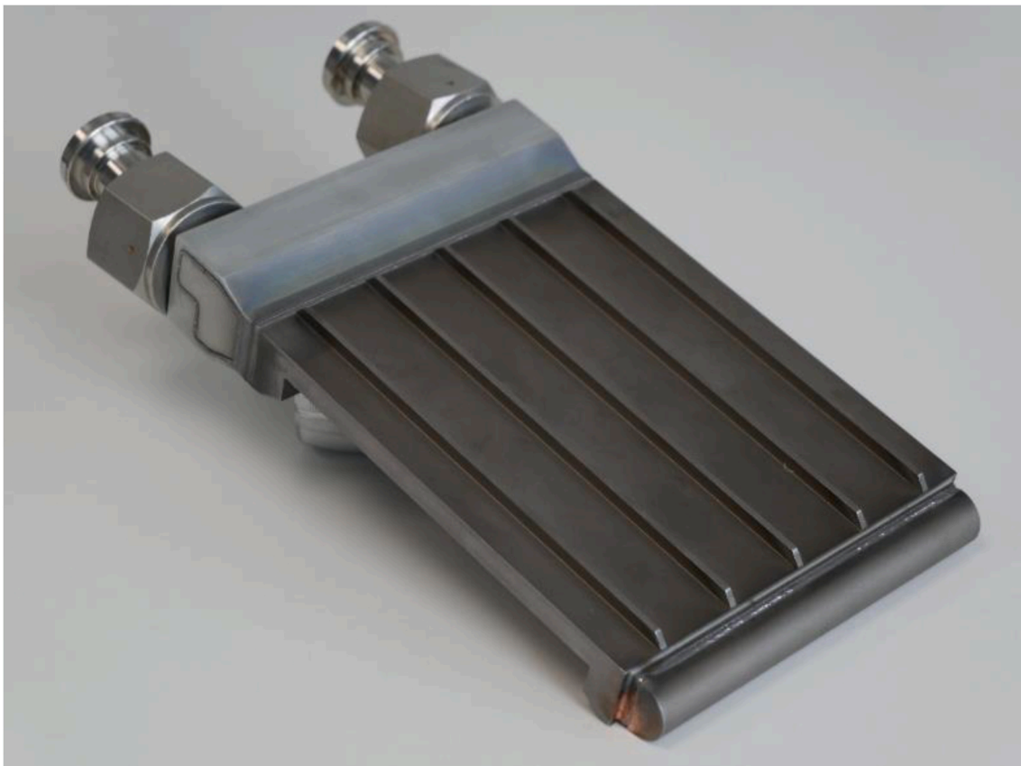
Fig. 29. Final manufactured HBS tantalum Target prototype (backside)
