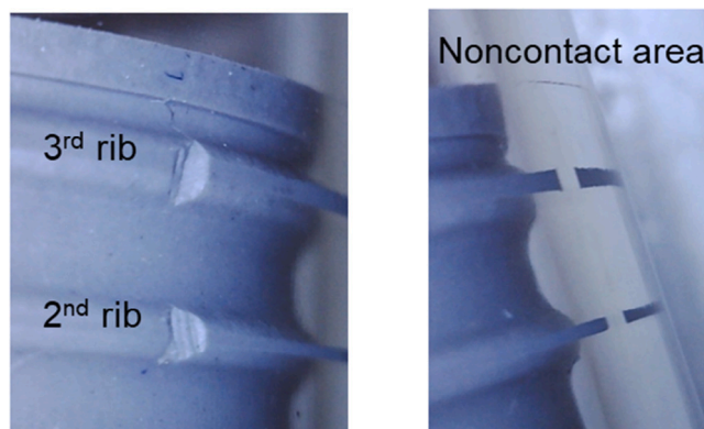
Fig. 8. Cuts and corresponding non-contact areas on the second and third ribs. The cuts were not large enough to significantly alter the contact pressure but were sufficient to allow air to pass through.
