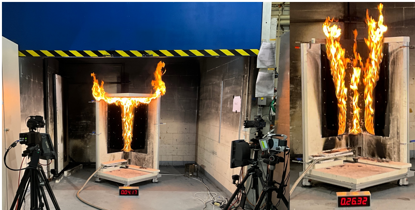
Figure 1. Experiment set-up, left: with ceiling, right: without ceiling.
