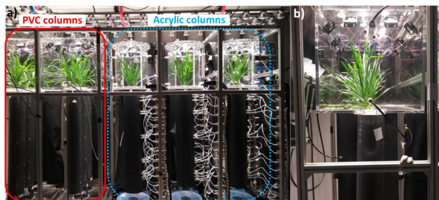
Fig. 1 Experimental setup of the columns in the climate chamber (a) showing the PVC columns (red) used for carbon, nitrogen and microbial analysis and the MRI root scans in this experiment and the acrylic columns (blue) which were used to determine root water uptake by Le Gall et al. (in press). Airtight chamber (b) used for ^{13}\text{CO}_2 pulse labelling of the plants
