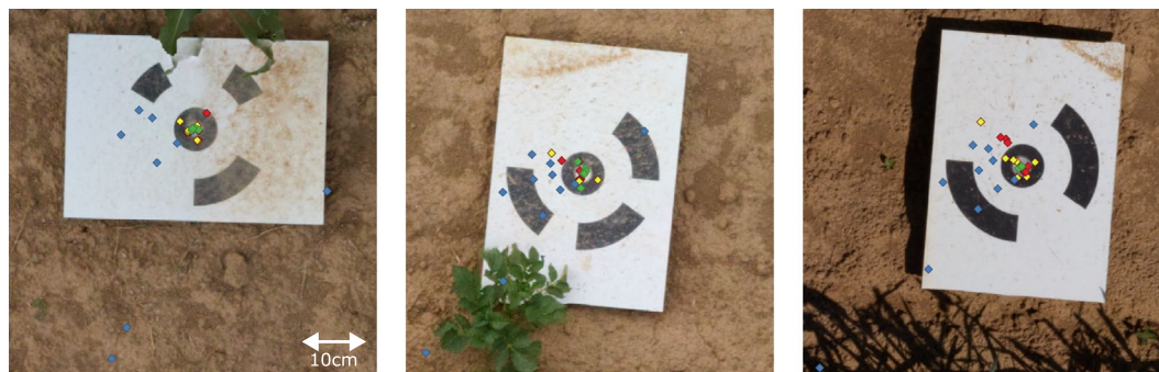
Fig. 11 GCP locations of UAV1-RGB (green), UAV2-RGB (blue), UAV3-RGB (yellow), and UAV3-MS (red), for each data collection date where the GCPs are visible. The GCP locations in the orthophotos are mostly aligned across sensors and different collection dates.
