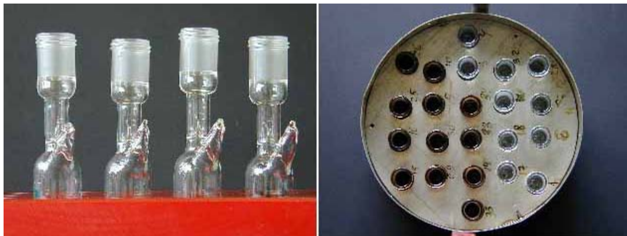
Figure 13. Glass tubes used for experiments in MTR cooling pool (left) and container with glass tubes (right)
