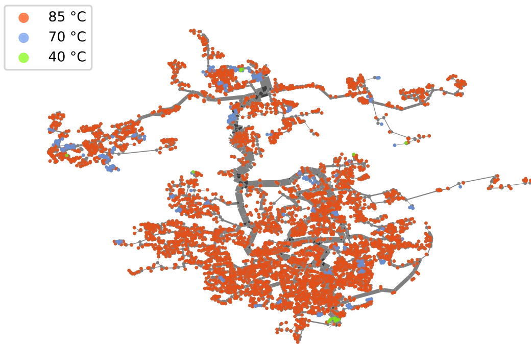
Fig. D.17. DH network of Essen including the maximum temperature requirements assumed at the heating systems of the supplied buildings.
