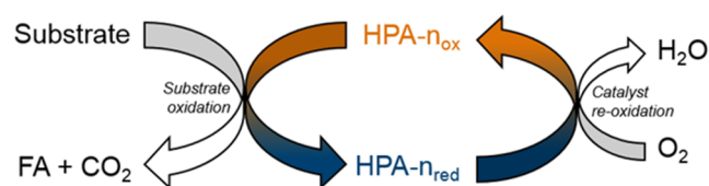
Figure 5. General catalytic scheme of the OxFA process divided into substrate oxidation (left) and catalyst reoxidation (right). 24
