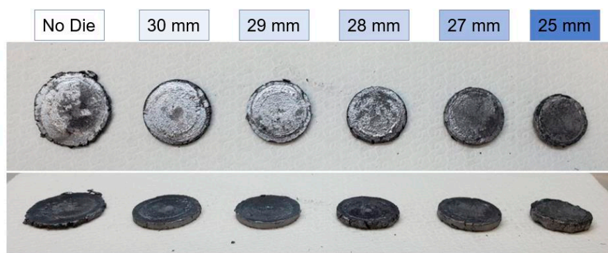
Fig. 4. Photo of the samples deformed via flash SPS with and without boron nitride dies
