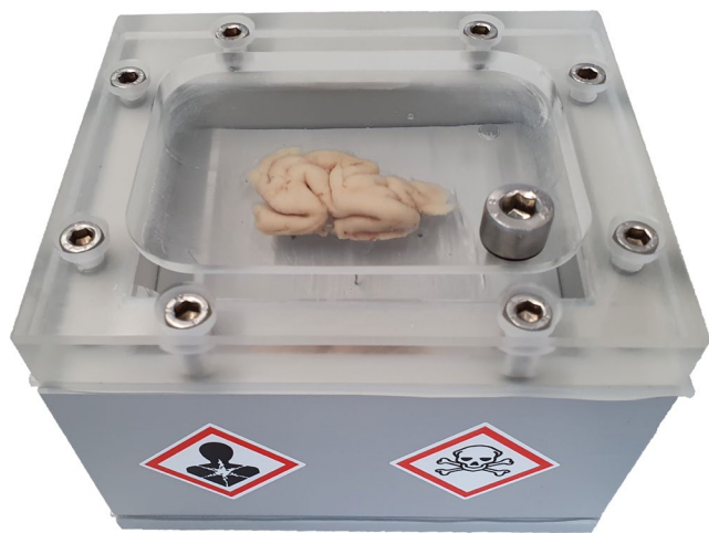
Fig. 2 Acrylamide embedding chamber. The chamber has a screwable lid and bottom, sealed by silicone sheets. The lid has an overflow tray, allowing the chamber to be filled without air bubbles via a filler neck. The filler neck is closed with a screw and a rubber seal. The volume of the chamber can be varied via plastic inserts. Blunt thin metal pins in the uppermost insert provide a separation to the bottom of the chamber. This ensures that the tissue is suspended in the acrylamide-solution and that it is completely embedded inside the hydrogel after polymerization
