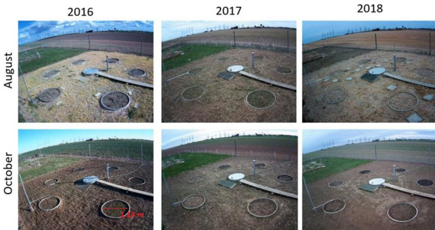
Figure 2-1: The lysimeters arranged in a hexagonal pattern at site SE3 at the start and end of the bare soil observation period for the years 2016–2018.
