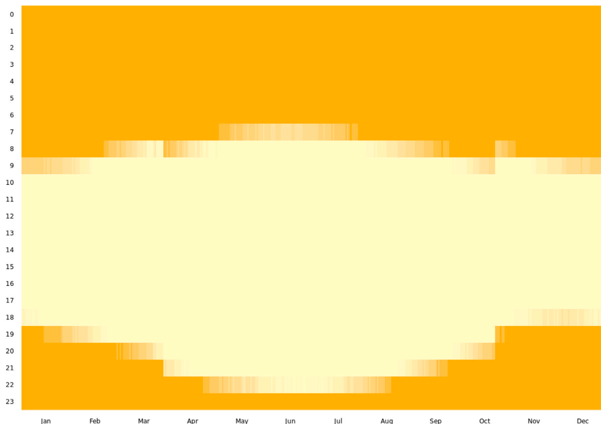
Fig. 11. Heatmap of Street Lighting (cluster 40), displaying night-time operation with seasonal adjustment to daylight hours.
