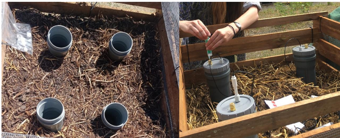
Figure A.6 Four static PVC tubes for periodic gas sampling with a syringe (right).
