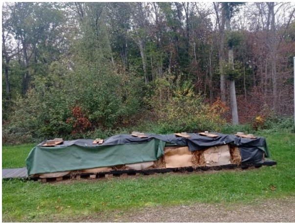
Figure A.5 Compost boxes with compost fleece, straw insulation and pond liner.
