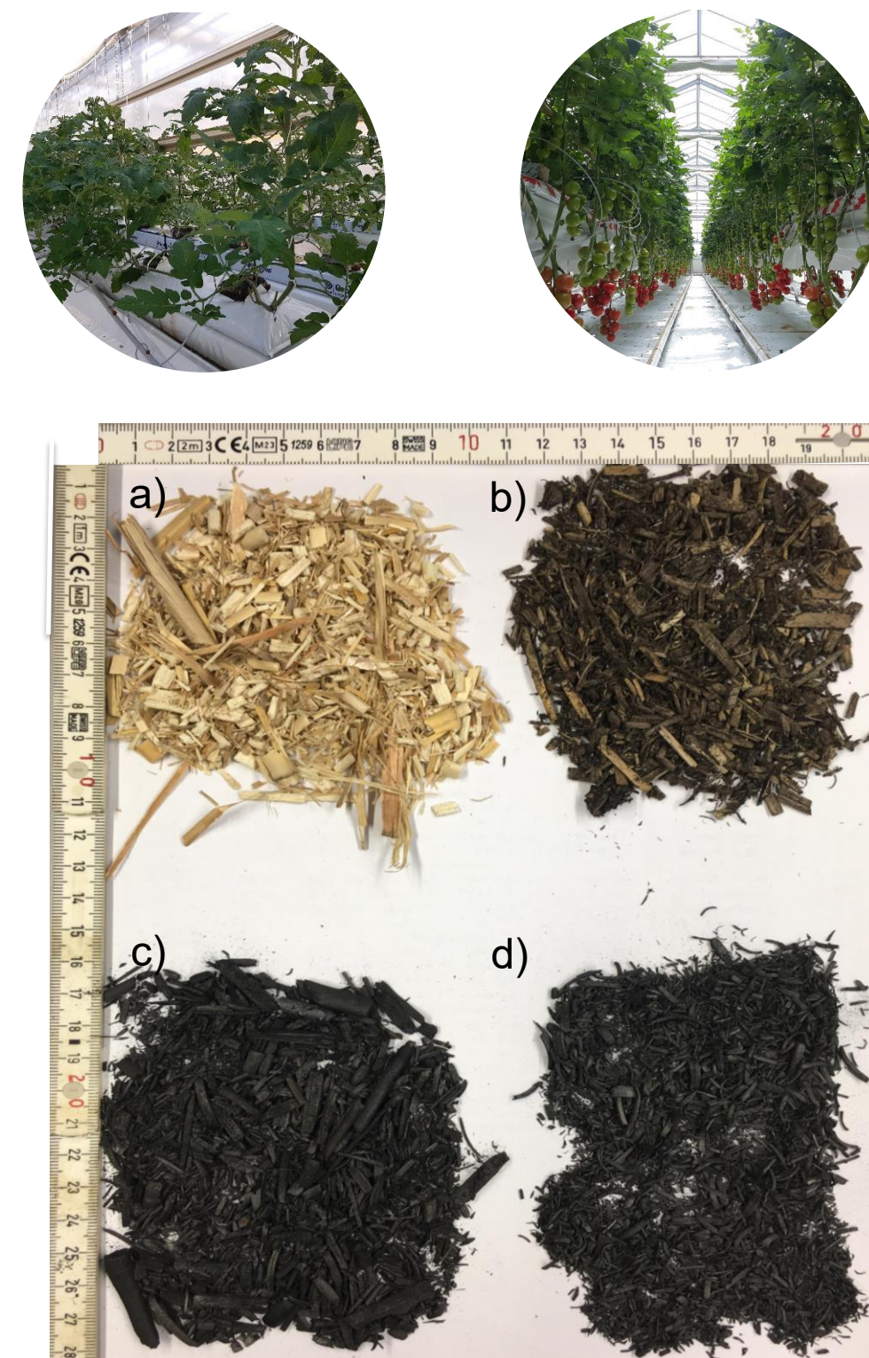
Figure 1. Illustration of fresh miscanthus (a), miscanthus substrate used 1x (b), biochar from fresh miscanthus (c) and biochar from miscanthus substrate used 1x (d).
