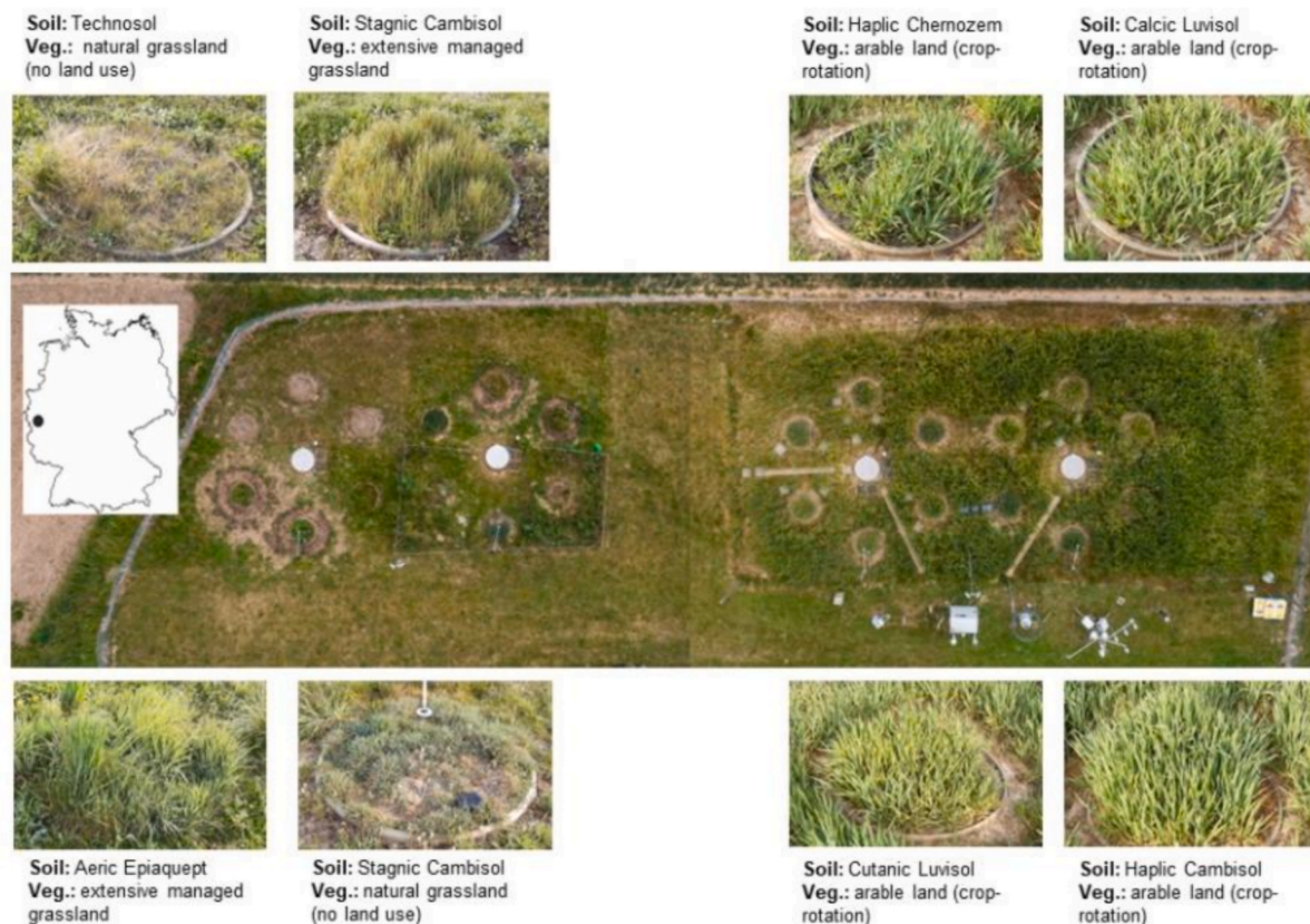
Fig. 1. Experimental set-up at the site Selhausen (Germany), showing the 24 high-precision weighing lysimeter and the information on the soil type, land cover form and management of the eight different agricultural ecosystems.
