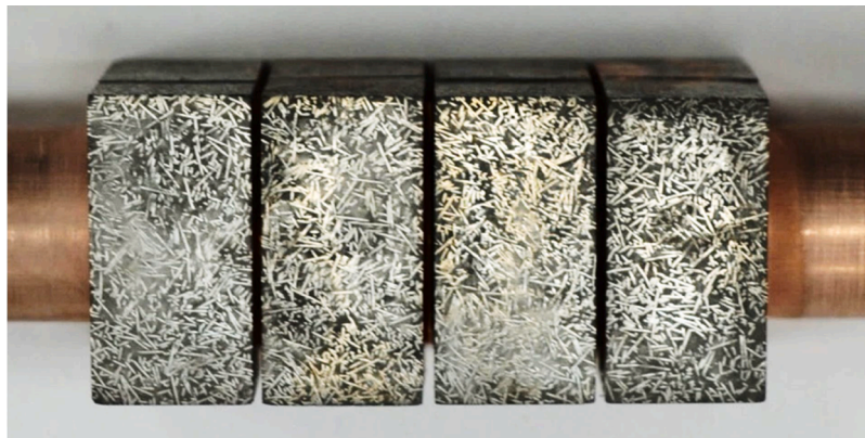
Fig. 14. HHF side of Wf/W blocks for mock-up ENEA 91.
