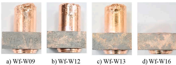
Fig. 9. Wf/W-Cu blocks after OFE-Cu casting.
