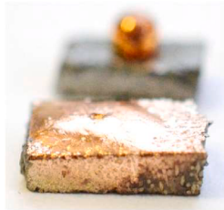
Fig. 7. Short-fibers Wf/W specimens #2 and #4 after Cu wettability test.
