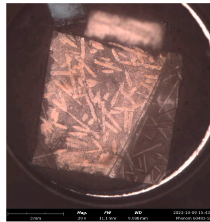
a) Optical image of a Wf/W specimen with dimensions 7x7 mm.
