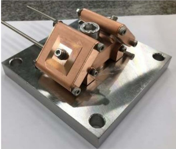
Figure 5. A two-axis coil prototype (55.AL) about to undergo thermal and vibration tests. Bolts through the LTCC sensors, in combination with copper foam ensure the in-vacuo heat transfer to the main block representing the ITER divertor. Frequency response is a few tens of Hz.
