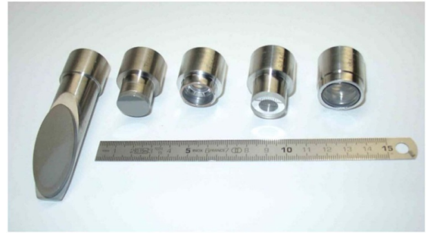
Figure 155. Brazed prototype window assemblies, UKAEA design.
