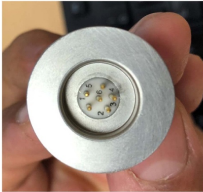
Figure 156. Example of ITER electrical feedthroughs with borosilicate GTMS inserts.
