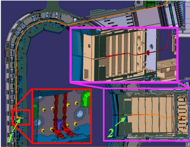
Figure 150. HFSR in-vessel layout in upper and equatorial ports of section #8. 1—HFS reflectometer antenna system; 2—Transmitting refractometry antenna.
