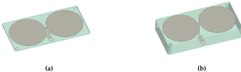
Figure 8. Antenna models with different PCB thickness: (a) h=1.5 mm, (b) h=10 mm.
