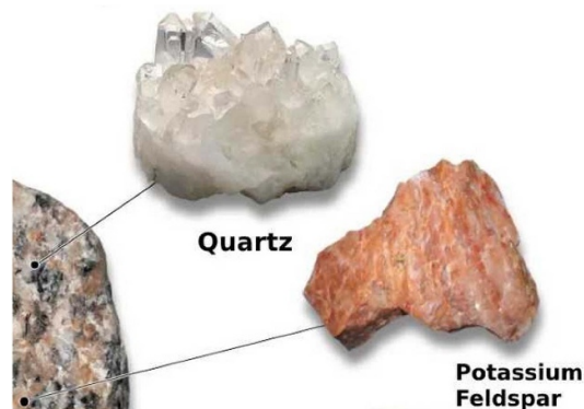
Figure 3. Granite consist of several minerals but the largest fractions are quartz and feldspar. Our granite looks visually similar to granite whose composition has been studied in detail, with \approx 72\% quartz and \approx 15\% feldspar.
