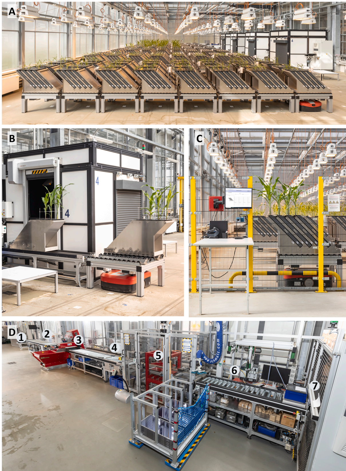
Fig. 1. GrowScreen-Rhizo 3 platform. A) Overview of the greenhouse compartment with 112 tables in the plant cultivation area in the center and four measurement chambers at the right side. One of the five red AGVs is visible below the front right table. B) Measurement chamber with a table in front, one magazine remaining on the table waiting for imaging and the second magazine on the conveyor in front of the chamber with one rhizotron pulled into the chamber. C) One of three presentation stations for sowing, manual measurements, and shoot harvest. D) Semi-automated filling line for rhizotron filling and root harvest. The labels in subfigure D mark the different stations of the filling line and are explained in the Material and Methods.
