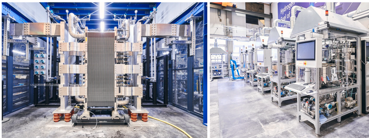
Figure 1. Test field environment used in DERIEL MW stack test bench (left) and kW stack test benches (right) (copyright by Siemens Energy)
